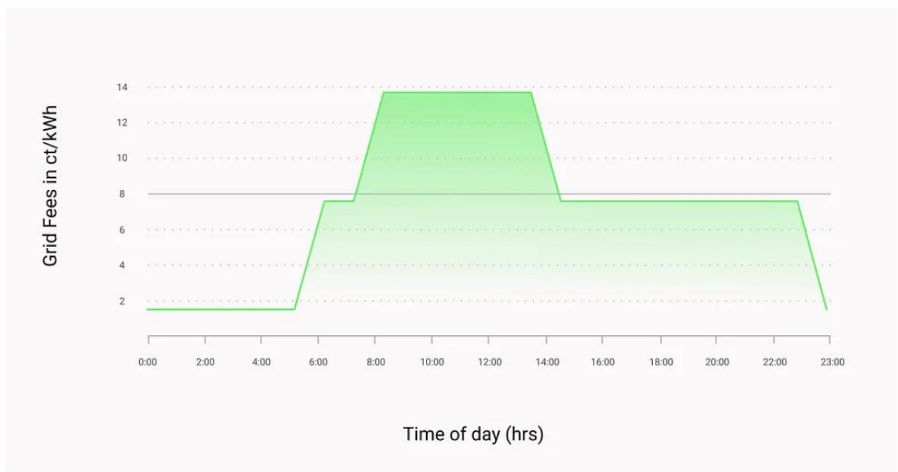
Figure 3. Graph of Time of Day Grid Fee Model, Grid Singularity Simulation of Germany 2030 Energy Market
