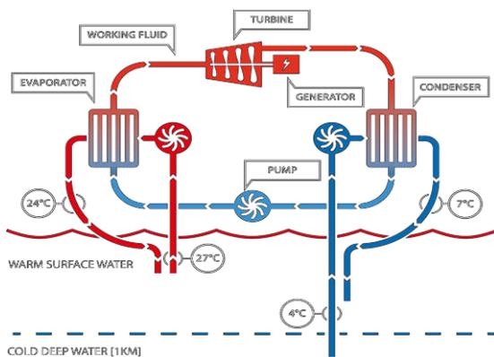
Figure 2 - Ocean Thermal Energy Conversion Cycle
