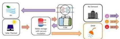
In summer operation (see Figure below left), the thermo-chemical material (TCM) storage can also provide cooling if required. The cold production matches with a discharge of the TCM storage. Charging of the TCM storage before the heating season will occur either in autumn or, thanks to the integrated buffer tank, during summer nights. In winter (see Figure below right), the TCM storage is designed to supply space heating demands for at least 4 weeks.
